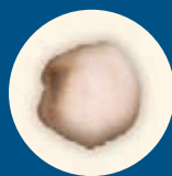
actual 8 micron dust particle magnified 1,500 times
